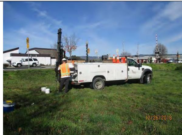
Placing liner in probe at boring SB-7.
