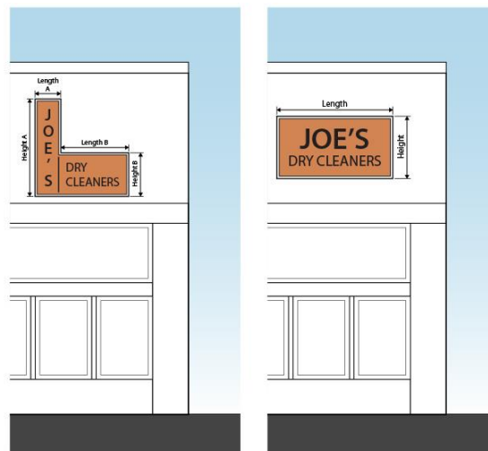
Figure 17.55-13 General Sign Area Measurement
