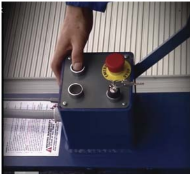
Key operated safety interlock switch at each unit
