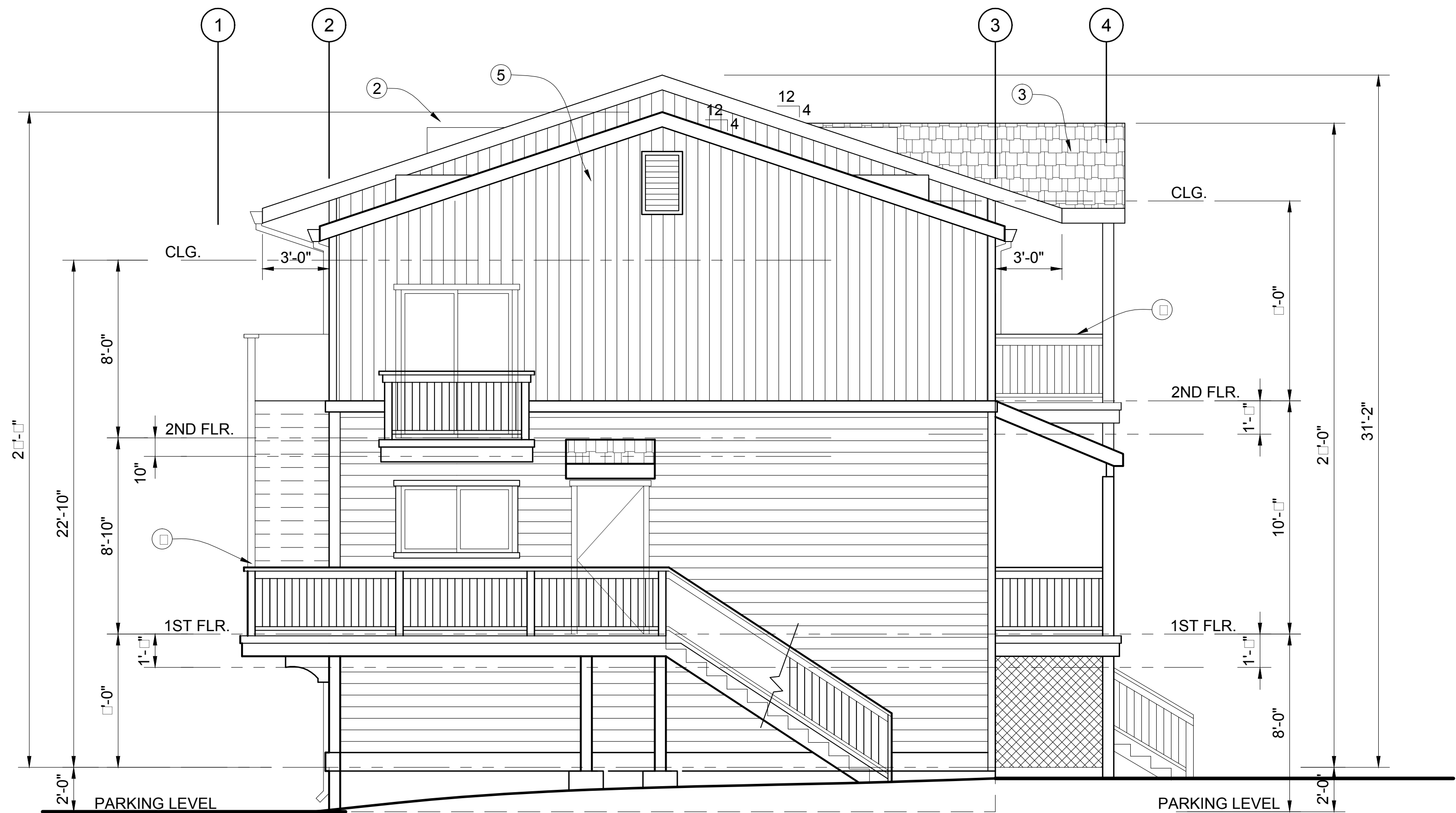
B PROPOSED SOUTH ELEVATION BUILDING 2 NORTH ELEVATION BUILDING 2 (SIM) SCALE: 1/4" = 1'-0"
