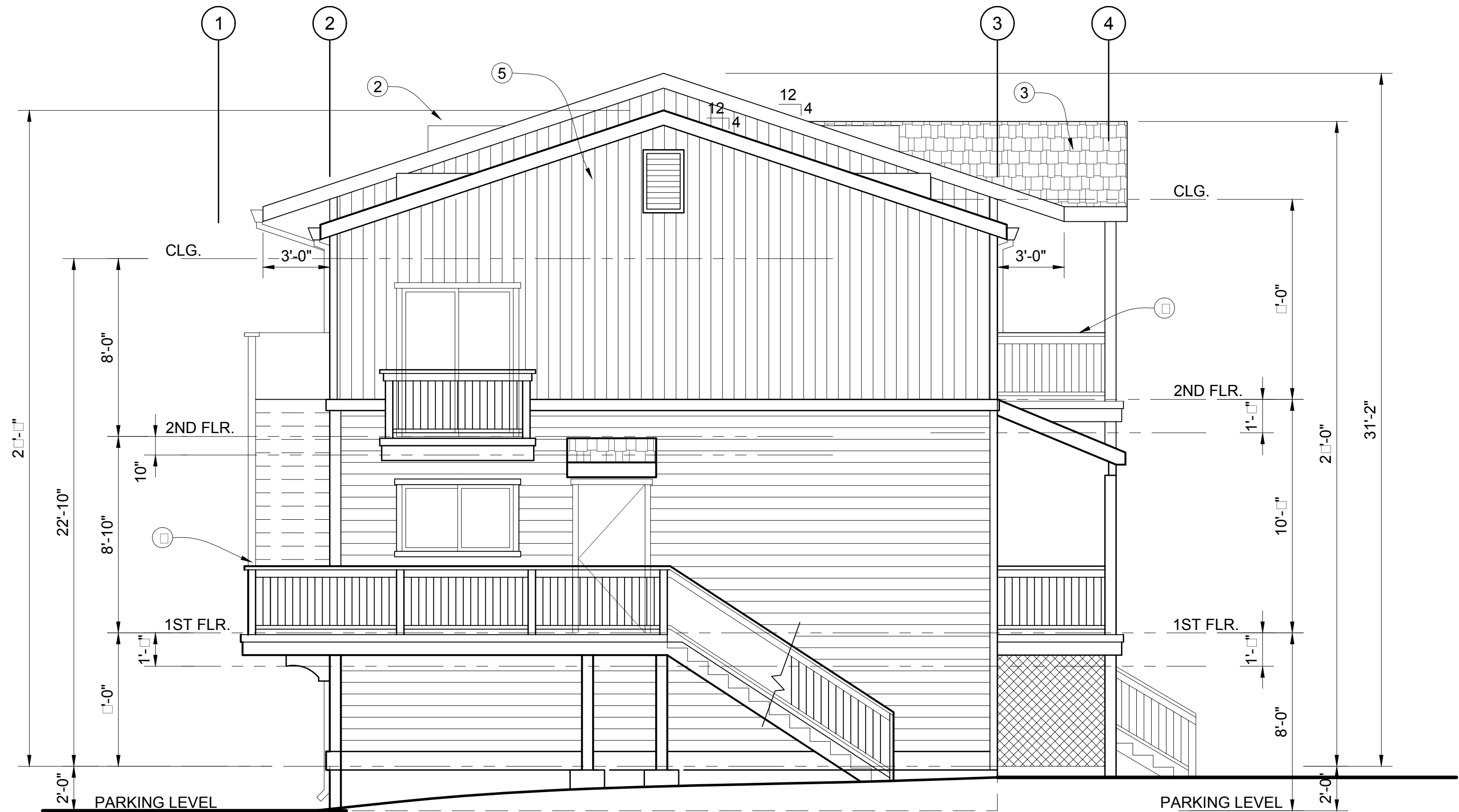
A PROPOSED EAST ELEVATION BUILDING 5 (SIM) WEST ELEVATION BUILDING 5 (SIM) SCALE: 1/4" = 1'-0"
