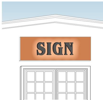
Figure 17.55-11 Reverse Channel Letter Sign
