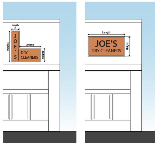
Figure 17.55-13 General Sign Area Measurement
