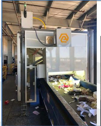
Left: recently installed 2<sup>nd</sup> "sorting" robot
