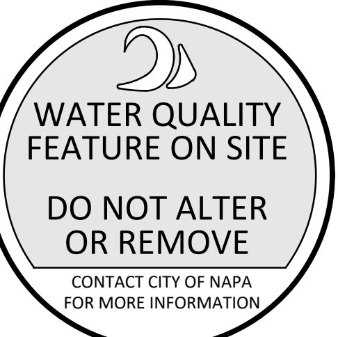
3 TM9 BIORETENTION FACILITY MARKER NOT TO SCALE
